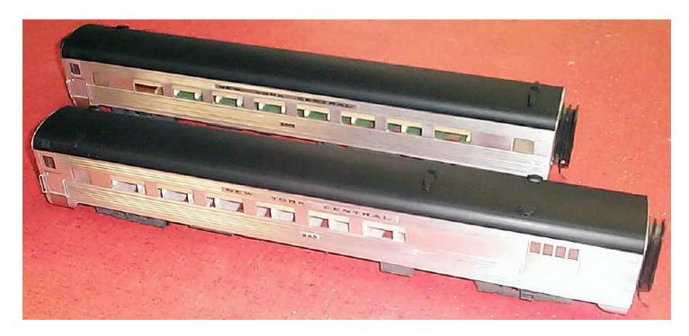
KASINER Kit 3 (coach) and Kit 6 (baggage / coach), in late 1950's New York Central pool service livery. These two kits were modified by shortening them to a scale 75' length in 1978, for operation on a small O scale layout. The under bodies have scratch-built Carrier air conditioning units, per their prototypes. The trucks and under body were painted Floquil Grimy Black. The roof was done with satin finish black Rustoleum spray paint. Champion decals were used for the lettering.
