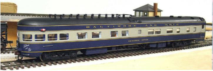
KASINER Kit 8, Pullman plan 4082 smooth side, 2 DBR/1 CPT/1 DRM/Observation Lounge built as B&O GENESEE RIVER. This model was built in 2006 from a \$10 'junker' car found on E-Bay. The vestibule doors of smooth side kits only had punched windows. The door openings on this model were marked off by scribing their outlines on the car sides and adding thin black stripe decals to better show the doors after the body was painted. Scale Coat paint and Micro Scale decals were used to finish this model.
