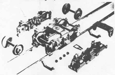
Due to the extremely close tolerances to which these trucks have been built, extreme care must be taken to have them fit together. If two parts do not fit, do not force them. Recheck the instructions.
