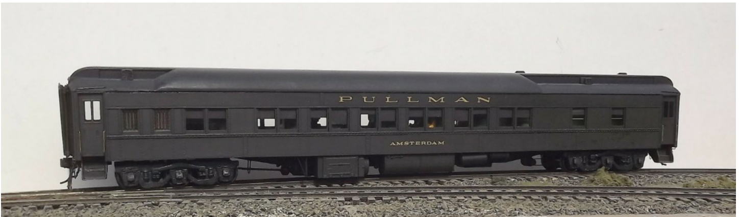
AMERICAN STANDARD KIT 3410: PULLMAN PLAN 3410 B, LOT 6351, 12 SECTION / 1 DRAWING ROOM SLEEPER. THE PROTOTYPE "AMSTERDAM" WAS AMONG THE LAST HEAVYWEIGHT SLEEPERS OUTSHOPPED WITH AIR CONDITIONING BETWEEN JANUARY AND FEBRUARY 1930. IT WAS A PULLMAN OWNED CAR REMAINING IN PULLMAN GREEN PAINT WHILE ASSIGNED TO THE B&O 1949-1956.
